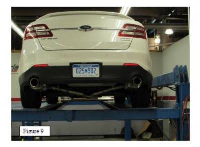
STEP: 11 Once the position has been determined to be correct, tighten the Accuseal™ clamp to 32-35 ft. lbs. making sure the clamp's openings are not over any of the notches in the pipes.
