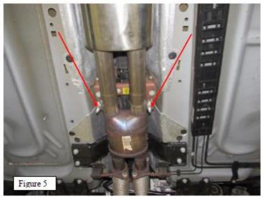
Step 7: Place two clamps over the expanded end of the intermediate pipe assembly. Install the intermediate pipes over the front muffler assembly making sure to install the hangers into the rubber isolators. (See Fig.6)
