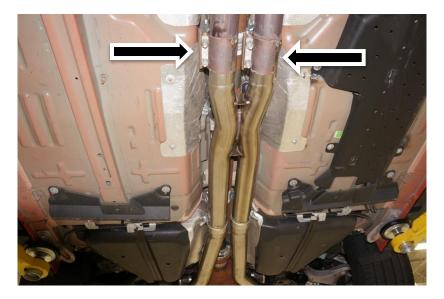
**10.** Install the X-Pipe with the short tails towards the front of the Vehicle using the Stock Exhaust Clamps. Loosely tighten the four (4) Nuts to allow for adjustment later.
