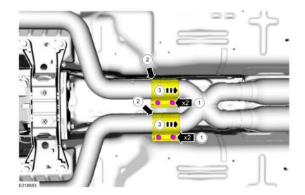
Loosen the <u>LH</u> and <u>RH</u> clamp nuts. *Torque*: **35 lb. (48 Nm)**
