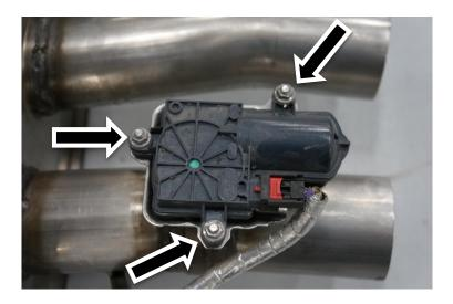
Remove the Exhaust Valve Actuators by removing the three (3) mounting Nuts and lifting the Actuator off of the Valve. DO NOT PRY THEM OFF. Transfer them over to the new Mufflers. Left to Left, Right to Right. *Torque: 3.0 Nm. +/- .3*
