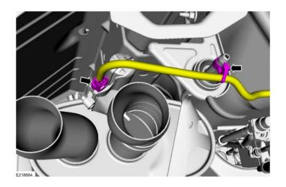
6. Disconnect the <u>LH</u> and <u>RH</u> tailpipe actuator electrical connectors. Detach the wiring retainers.
