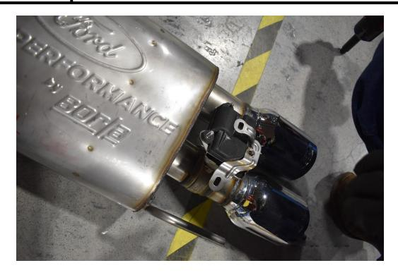
Step 5: Install supplied clamps onto the new muffler inlets and slide muffler hangers into factory exhaust hangers. Next slide the mufflers over the under axle pipes, centering tips in rear bumper opening. Attach the wiring harness to the valves if applicable.
