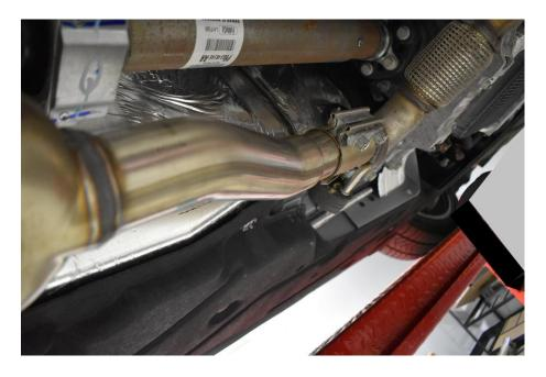
Step 2: Install factory hangers (previously removed) onto under axle pipes.
