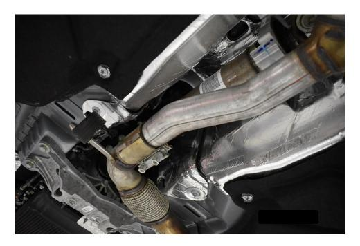
STEP 5: Using a 13mm socket to remove bolts from exhaust hangers in rear Sub frame near the rear axle, LH and RH sides.
