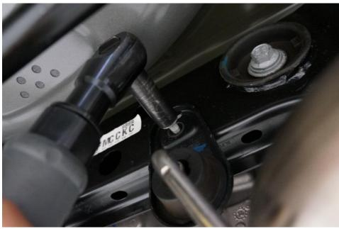
Step 4: Using a 13mm socket tighten bolts to 25 nm (18 lb-ft) in rear Sub frame exhaust hangers.
