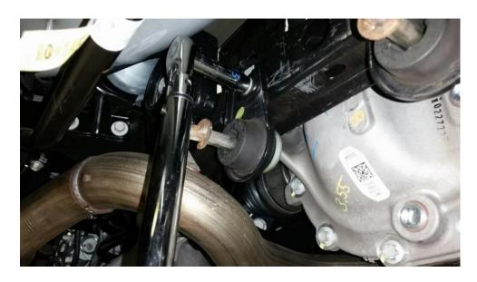
NOTE: For systems with valves, the actuator will have to be removed from the factory system by removing 3 nuts as shown and attached to the valve on the new exhaust. The Factory bracket also needs to be installed in the factory location.
