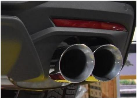
Step 6: Check your exhaust system for proper clearance under the vehicle and also for tip alignment, tighten the clamps to 32-35 ft. lbs, checking tip alignment and clearances as you do. There should be a minimum gap of 25mm from the tips to the edge of the car, and the tips should be in 25mm from the outermost edge of the rear bumper.
