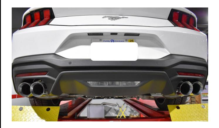
STEP 7: Lower vehicle. Start vehicle and check for any leaks. If any leaks are found, determine cause (such as loose or incorrectly positioned clamp) and repair as necessary.
