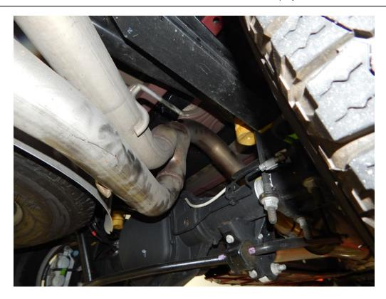
STEP 4: Install the rear-most isolator removed earlier, sliding it over the hanger of the tailpipe assembly. Torque the bolts to 22 ft-lbs (30 N-m).
