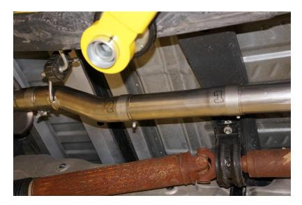
Step 4: Install the mid-muffler onto the hanger and slip into S-pipe.
