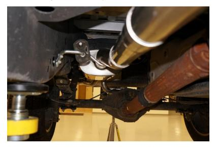
Step 6: Slide (2) 2.25" clamps over the muffler outlet pipes. Work the tailpipe assembly past the spare tire and suspension, then onto the muffler outlet pipes. Push the most forward hanger into the factory rubber isolator, then push the rearward hanger through the factory rubber isolator. Slide clamps into proper position on the joints, then snug, do not tighten.
