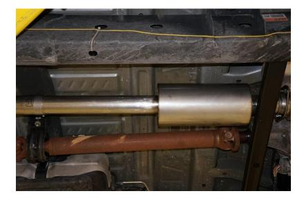
STEP 2: Install the proper "Mid Pipe" for your wheel base. Be sure to slip a clamp onto the pipe, clamp to be tighten later.
