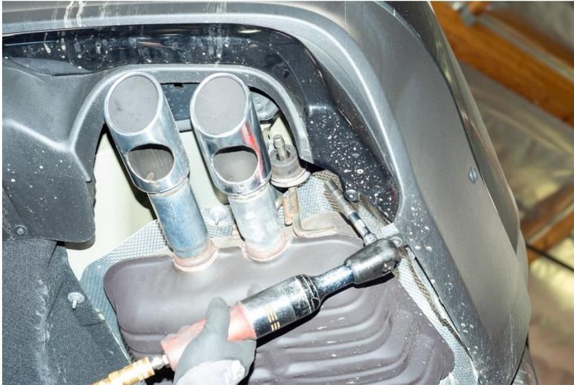
**STEP 3:** Remove the under-axle hanger brackets from the frame, retain the hardware.
