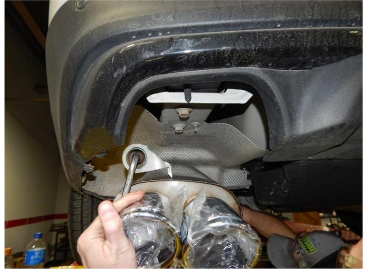
**STEP 4:** Center the tips in the cutouts. Check your exhaust system for proper clearance under the vehicle. Tighten the clamp to 32-35 ft. lbs, checking the tip alignment and clearances as you go.
