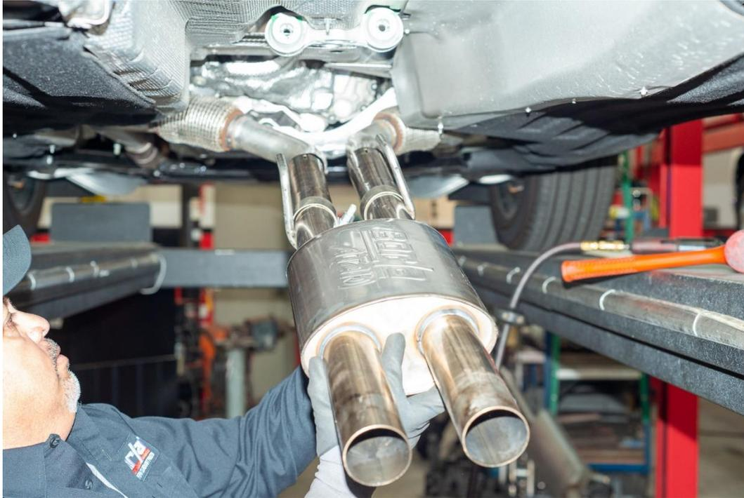
**STEP 2:** Place a clamp over the expanded inlet of the under-axle pipe, then slide it over the muffler outlet. Slide the hanger bracket over the hanger and attach to the body. Do not tighten the clamp. Repeat for the other side.
