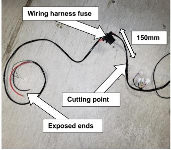
52. With the wiring harness 180409, measure and cut the red and black wire 150mm from the fuse.
