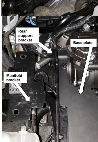
49. Loosen the factory flange bolt from step 8, and rotate rear support bracket, and place between the base plate and DLCM.
