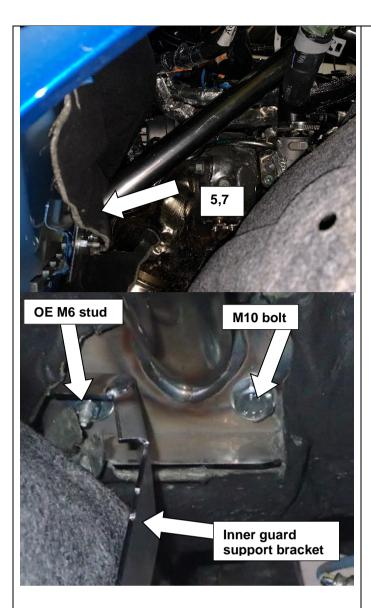
5. Feed support tube weldment to the firewall and locate onto the M6 stud. Once on, place the inner guard support bracket over the same OE factory stud, and fasten OE M6 nut.
