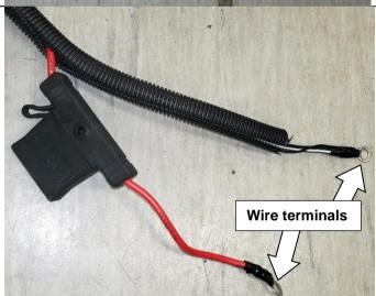
54. Crimp a terminal to the end of each of the two wires on the compressor wiring harness (pn 180409).
