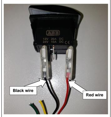
63. Connect spade connectors (from step 55) to the switch pins as follows:
