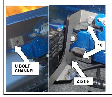
9. Feed the U BOLT CHANNEL behind the chassis from the top
