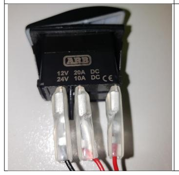
64. Connect the spade connector (from step 62) to switch pin 2.
