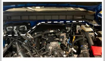
60. Pickup power from the stability bar module fuse (10A) located in the engine bay fuse box. Fuse reference #158 in owners manual.
