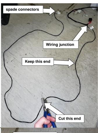
51. Using the wiring harness 180409, measure (from the junction) and cut the green/red/yellow/black wire to a length of 750mm (cut end with spade connectors).
