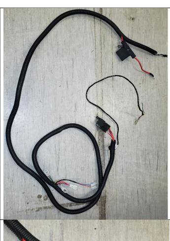
53. With the two cut sections of the wiring harness, reverse and reattach (the section with the fuse) by soldering the exposed ends to the ends of the other section that were cut in the previous step.
