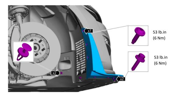
2. Remove the 4 belly underbody shield covers
