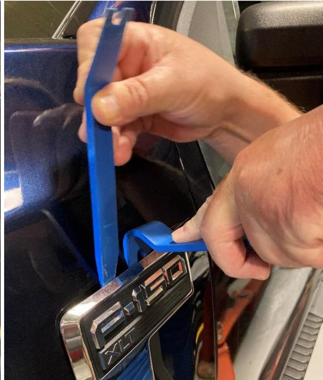
2. If the clips remained in the slots on the fender, remove old clips before installing new fender vent.
