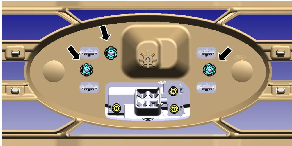
10. Use a T25 to remove the (3) M5 screws
