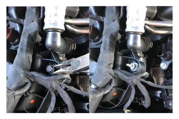
Step 3. Install one 8mm self-locking nut on stud bolt. This will be used as a spacer for the bracket.
