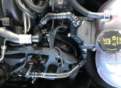
Step 7. Reinstall engine cover (and strut tower brace if taken off. Torque to 60Nm)
