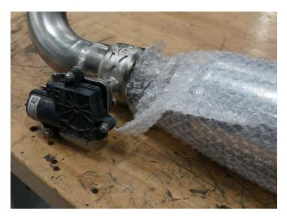
Transfer the Exhaust Valve from the factory exhaust to the new system by removing the three 8mm nuts. Be sure the exhaust valve is positioned to match up to the valve motor.
